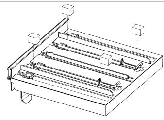
Remove adhesive backing from both sides of foam tape pads. Place foam tape pads onto pusher tray.
