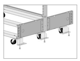
Attach caster assemblies to the end bottom arms by aligning the outside hole on the caster assembly with the hole in the bottom arm and secure with 1 5/16 X 3/4 bolt per bottom arm.
