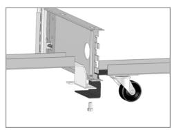
Attach the starter caster assembly and the add on caster assembly by overlapping them under the center bottom arm as pictured above and secure with 15/16 X 3/4 bolt per bottom arm.
