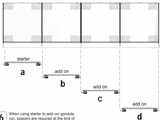
When using starter to add–on gondola run, spacers are required at the end of the run as pictured above. Refer to step 2 for installation.
