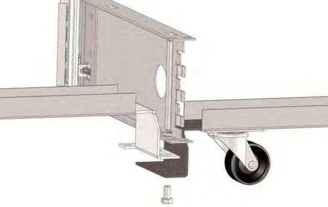
When connecting a <u>starter to a add-on</u> <u>unit</u> no spacer is required. Just slide the casters one above another as pictured above and bolt together
