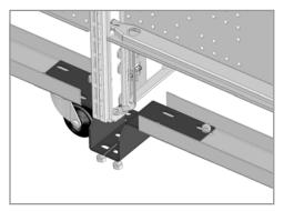
Attach caster assemblies to end and center standards by aligning the inner–most hole on the caster asembly with the hole in the bottom and the standards and secure it with 1 5/16 X 3/4 bolt per end of caster assembly.
