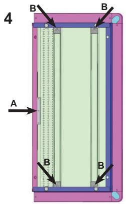
Center the Deck and the base assembly. First, fasten the deck the back kick with one (1) Tek screw. Fasten each (4) mounting clip to the deck hat with one (1) Tek screw.
