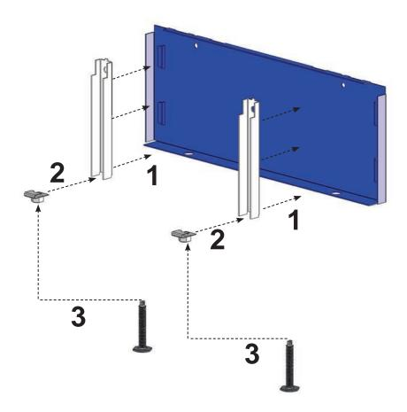
Tilt the leveler channel into the side channels as pictured above. Slide the U-Channel over the side lip so it retains the leveler channel as pictured. Insert the leveler into the U-nut as pictured below.
