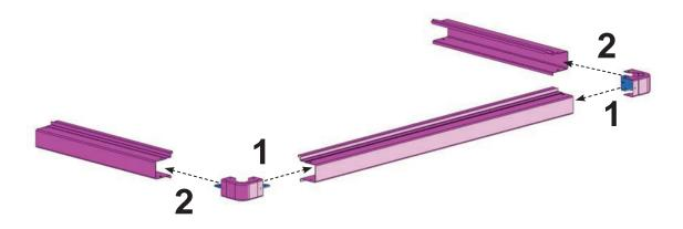
Slide the Trim Gurad fronts and side together as pictured above. When seated properly pre-drilled holes will align. Fasten the front and sides to the corners with four (4) Tek screws per side, two (2) Tek screws per side and front as pictured below.
