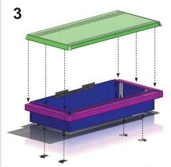
Set the deck on the base assembly and flip the entire assembly over. Set mounting clips on hats so each clip hooks the sides (Two (2) per hat as pictured to the right).
