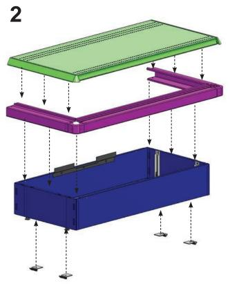
**OPTIONAL FEATURE:** Slide the assembled base nose (see page 2 for assembly) over the base assembly. Make sure all sides are seated.
