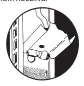
9) Install the back panel from step 4. Slide down from top...
