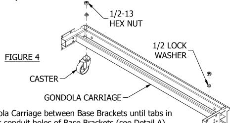
STEP 7: Slide assembled Mobile Gondola Carriage between Base Brackets until tabs in end plates fit into 2" diameter conduit holes of Base Brackets (see Detail A).
