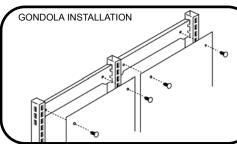
Using provided plastic fasteners, install the back stiffiner clips. The back stiffiner clips lock into the upright slots and are secured through the center of the backs. Make certain that the back stiffiner clip fastens **behind** the the back as shown at left.
