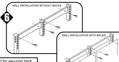
NOTE: Hardware is provided for securing back panels to bay stretchers. Installer must supply hardware for wall installation.
