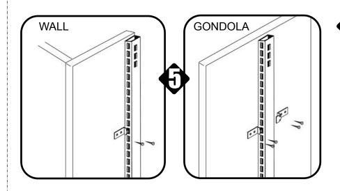
After the system has been plumbed and leveled, secure the uprights to the boxed corners, bay end boxes and end panels using the provided hardware. Bay uprights should be centered on double bay panels at 9 1/8" from the edges. Wall uprights will be flush with single bay panel edges.
