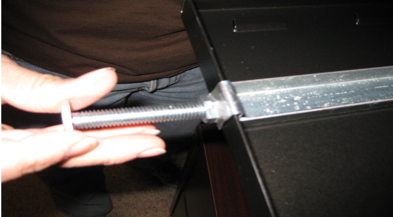
Screw leveler into nut. This will hold in place although some movement is felt.
